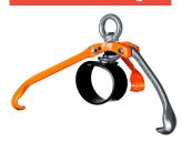
The REMA DG10 is an innovative patented invention for quickly and safely lifting 220 liters of steel and plastic drums with an edge diameter of 570 to 610 mm. The drums can be lifted both from standing and lying position. Furthermore, it is possible to lift a specific drum from the middle of a group of barrels.
